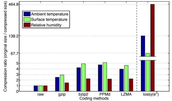
Fig. 13. Compression ratios of our archiving scheme compared with various lossless coding methods. Our scheme allows distortion up to the sensing accuracy.
