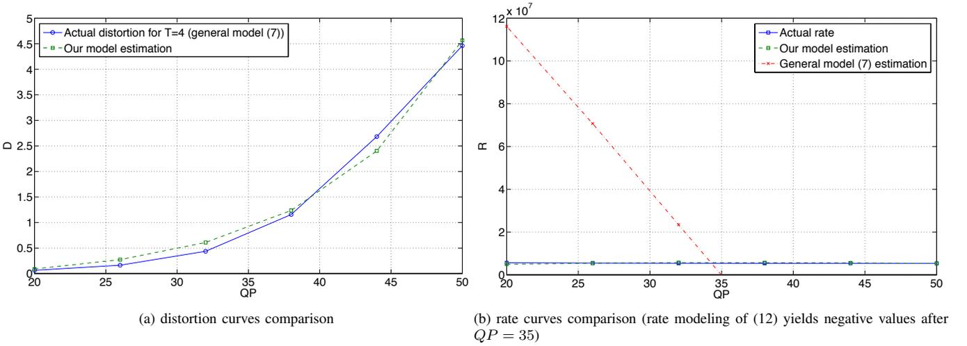
Fig. 11. Comparison of our model and general model with actual rate-distortion curves.
