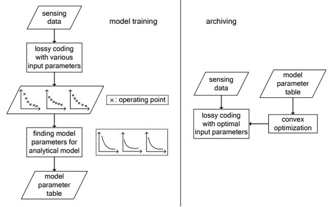
Fig. 1. Flowchart for optimal storage configuration. Each sensor data type has its own model parameter set.
