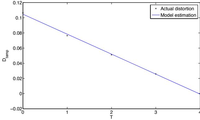
Fig. 9. Temporal distortion as a function of  $T$  estimated by (10).
