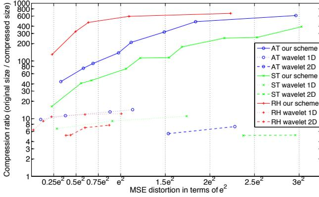
Fig. 14. Log-scale compression ratios of our archiving scheme compared with wavelet-based methods using partial correlations at various data fidelities in terms of the sensing accuracy. Acronyms are explained in Table I.
