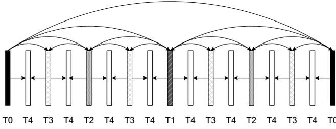
Fig. 4. Temporal coding and prediction structure of our spatio-temporal decorrelation module. Each increasing temporal level coincides with including collections of sensor data labeled the corresponding level, i.e.,  $T_i$ .
