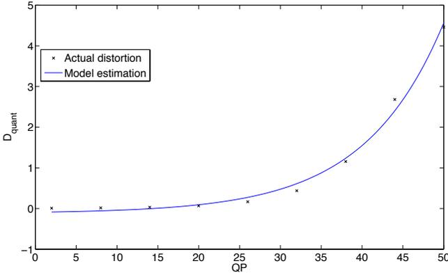
Fig. 7. Distortion curve as a function of  $QP$  estimated by (4).
