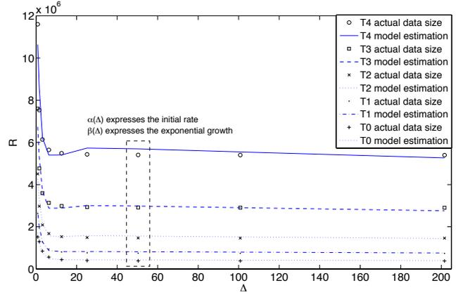
Fig. 5. Sizes of compressed data blocks  $R$  as functions of quantization step sizes  $\Delta$  for different temporal levels  $T$  estimated by (1).
