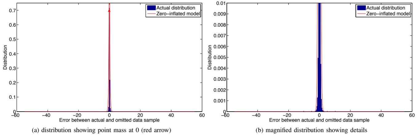
Fig. 16. Distribution of error fitted with zero-inflated Laplacian distribution.
