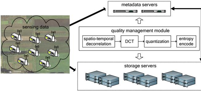
Fig. 2. Quality management module working with conventional distributed file system. Black arrows represent data and control flows of file system. Lossy coding runs on storage servers under control of metadata servers.
