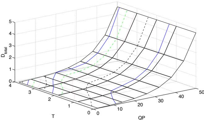
Fig. 12. Isolines of rate over distortion surface of ambient temperature  $T$ . Minimum distortion is obtained along the boundary of  $QP$  and  $T$ .
